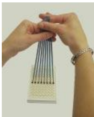
Figure 3: Performing Serial Dilution
